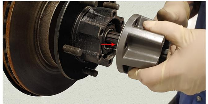
7. Reusing original fasteners, torque to specification. Reinstall Snap Ring (apply outward pressure to axle if necessary).
