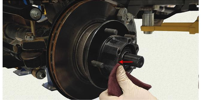
6. Lightly lube warn locking hub seal and install.
