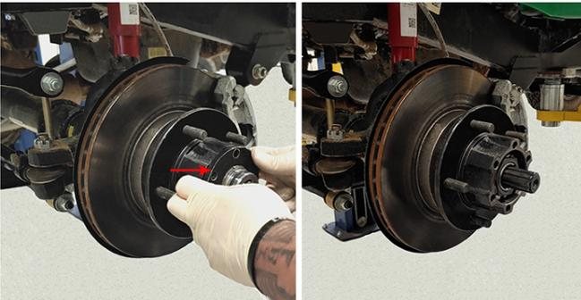
5. Clean sealing surface before installing new locking hub.
